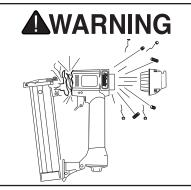
Exceeding the maximum permissible operating pressure may damage the nailer/stapler and cause it to malfunction. To protect yourself from personal injury, DO NOT allow the air pressure to exceed the recommended pressure for these tools!
